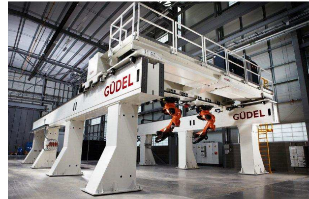
Large scale gantry system
